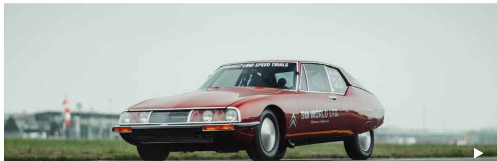
The record SM car, twin turbo did its record attempts nose down rear up for stability thus not needing any wings which would have slowed it down.
